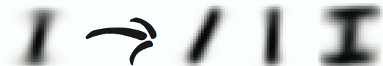
Figure 21: On the left, the AVERAGE of all 5600 samples in the I class and, on the right, the AVERAGE of each of the k -means clusters with k = 3 as performed under PCA . Wanting to ignore horizontal strokes for legibility reasons, I only train the neural network on samples from the first two clusters in order to guarantee a detected stem.
